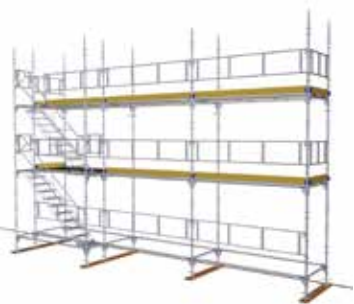
Independent Load classes 1 - 6 Bay width 700, 770, 1050, 1250, 1655 mm Decking: Decking unit, steel plank, aluminium plank
