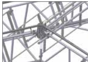
The fall protection anchor in place
